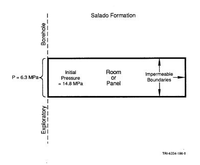
Figure 4-19. Schematic Diagram Showing Repository Region and Boundary Conditions for Evaluating Characteristic Depressurization Times.
