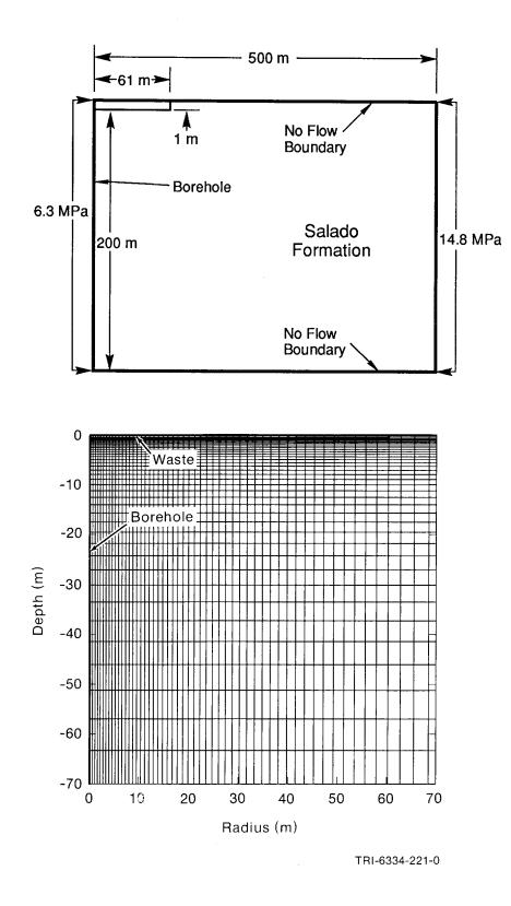
Figure 4-1. Boundary Conditions Applied in Borehole Model and Axisymmetric Mesh for SUTRA Calculations of an Intrusion Borehole through a Waste Panel.
