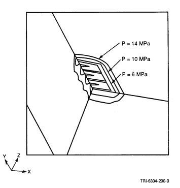
Figure 4-28. Pressure Contours Showing Very Little Pressure Disturbance about WIPP Quarter Panel after 10,000 Yr with Capacitance Equal to 5.1 x 10<sup>-9</sup> Pa<sup>-1</sup>.
