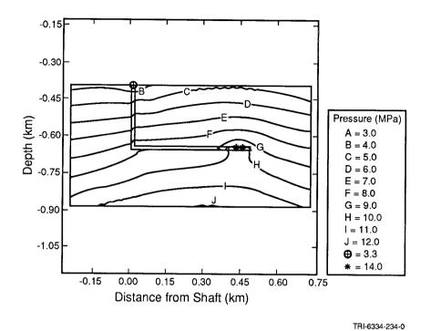
Figure 3-17. Pressure Contours for SUTRA, Set II, Case IA, with Expected Properties and Boundary Conditions Interpolated from Large-Scale Simulation at 10,000 Yr. (Figure 3-10 shows the corresponding large-scale simulation.)
