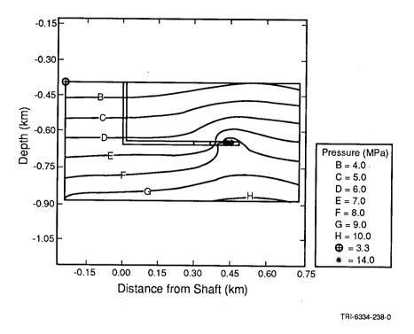
Figure 3-21. Pressure Contours for SUTRA, Set II, Case IC, No Shaft Seal at 10,000 Yr.
