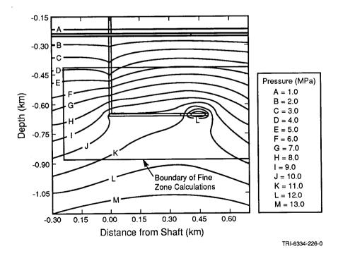
Figure 3-10. Pressure Contour Details for Large-Scale SUTRA Calculations Used to Provide Boundary Conditions for Set II, Case IA (Steady State).
