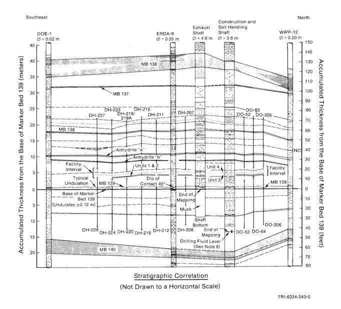
Figure 1-5. Marker Bed 139, One of Many Polyhalite Anhydrite Interbeds near the WIPP Repository Horizon.
