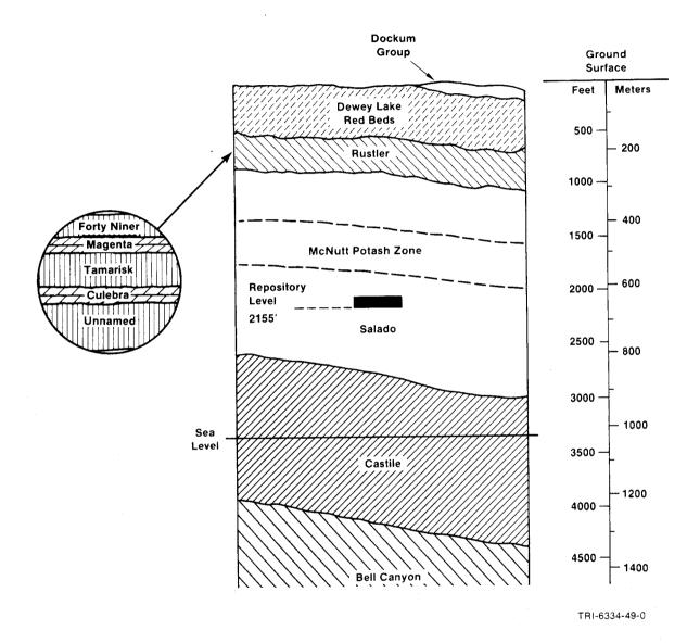
Figure 1-2. Level of WIPP Repository, Located in the Salado Formation. The Salado Formation is composed of thick halite with thin interbeds of clay and anhydrite deposited as marine evaporites about 255 million years ago (Permian period) (Rechard, 1989).
