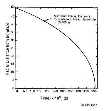
Figure 4-7. Radial Distance versus Time for Neutrally Buoyant Particle in Transient Velocity Field for Capacitance of 7.8 x 10<sup>-12</sup> Pa<sup>-1</sup> as Calculated by TRACKER.
