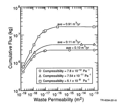
Figure 4-5. Variation of Cumulative Flux with Permeability at a Salado Formation Capacitance of  $5.1 \times 10^{-9}$  Pa<sup>-1</sup>, 7.54 x 10<sup>-11</sup> Pa<sup>-1</sup>, and 7.8 x 10<sup>-12</sup> Pa<sup>-1</sup>.
