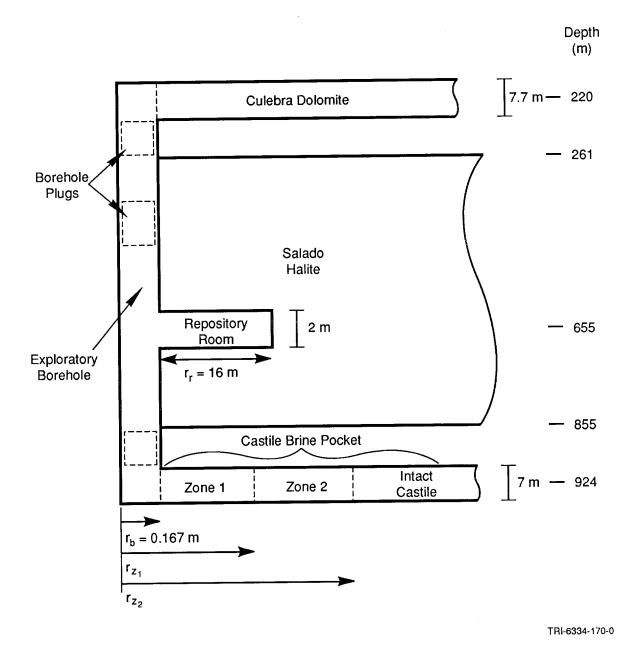
Figure 4-13. Schematic Diagram of the Geometry Used for Calculating Access Fraction from Brine Pocket Flow.
