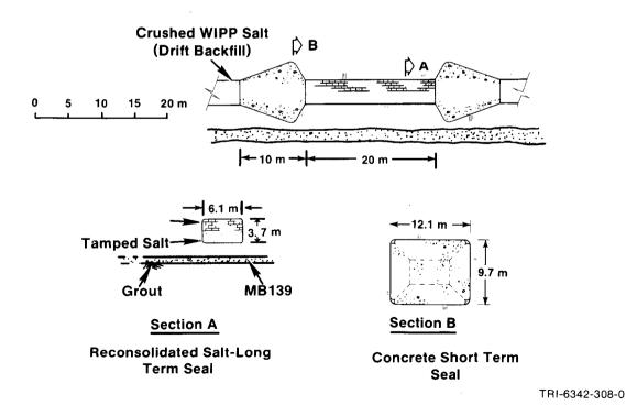
Figure 1-9. Schematic of Typical Multicomponent Seal for Drifts and Panels (after Nowak et al., 1990).
