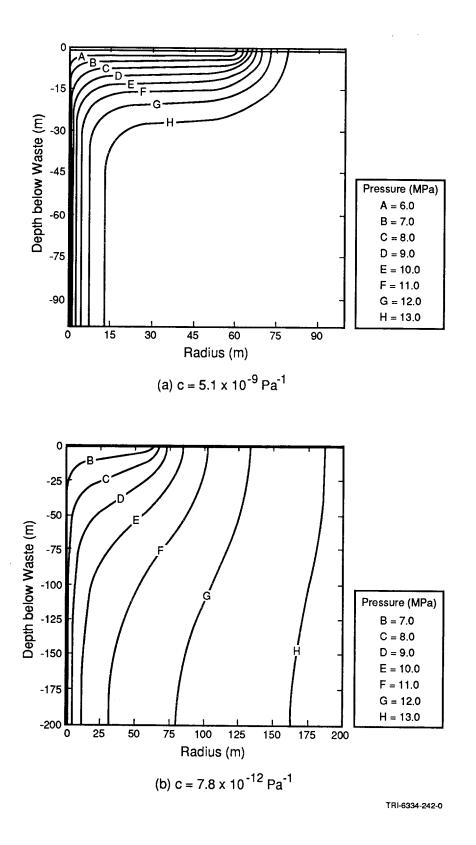
Figure 4-4. Pressure Contours near Cylindrical Waste Panel at 10,000 Yr for a Capacitance of (a) 5.1 x 10<sup>-9</sup> Pa<sup>-1</sup> and (b) 7.8 x 10<sup>-12</sup> Pa<sup>-1</sup>.
