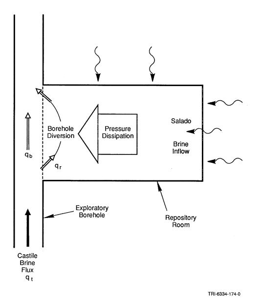
Figure 4-12. Conceptual Model of Repository Flow Field Considered in Calculation of Access Fraction from Brine Pocket Flow.
