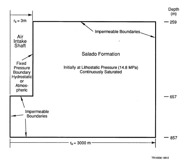
Figure 3-25. Schematic Diagram of Geometry and Boundary Conditions Used in the Air Intake Shaft Inflow Calculations.
