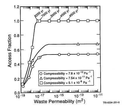
Figure 4-6. Variation of Fraction of Panel Accessed with Permeability at a Salado Formation Capacitance of  $5.1 \times 10^{-9}$  Pa<sup>-1</sup>, 7.54 x 10<sup>-11</sup> Pa<sup>-1</sup>, and 7.8 x 10<sup>-12</sup> Pa<sup>-1</sup>.
