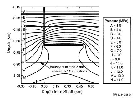
Figure 3-12. Pressure Contour Details for Large-Scale SUTRA Calculations Used to Provide Boundary Conditions for Set II, Case IB (Steady State).
