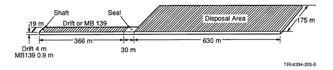
Figure 3-36. Model of Disposal Area, Seal, and Drift (or Marker Bed 139) Leading to Shaft (83 Blocks).
