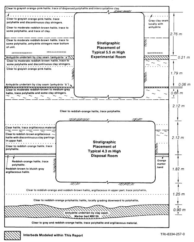
Figure 1-3. Stratigraphy at the Repository Horizon (after Lappin et al., 1989). Units in disposal area dip slightly to the south, but disposal excavations are always centered about the orange marker band (reddish-orange halite).
