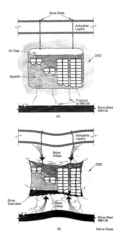
Figure 2-1. Hypothesized Episodes in Disposal Area Leading to Undisturbed Conditions. This drawing shows (a) initial conditions after decommissioning and (b) room creep closure and brine inflow.
