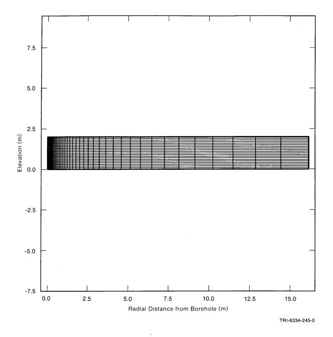
Figure 4-15. Model Grid and Boundary Condition Locations for Brine Pocket Calculation. Fixed-pressure boundaries were imposed at the top and bottom of the borehole.
