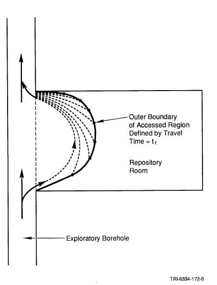
Figure 4-17. Schematic Diagram Illustrating the Region from which Soluble Species Will Be Removed by Flow from a Brine Pocket in Specified Time,  $t_r$ .
