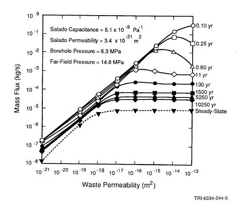
Figure 4-3. Variation of Transient Mass Flux to a Borehole as a Function of Waste Permeability.
