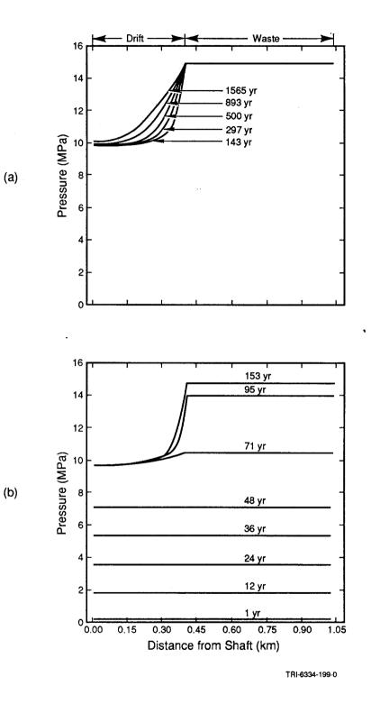
Figure 3-35. Gas Pressure Profile Without Seal and With Time-Dependent Drift and Waste Permeability, Calculation 5, (a) 142 to 1,565 Yr and (b) 1 to 153 Yr.
