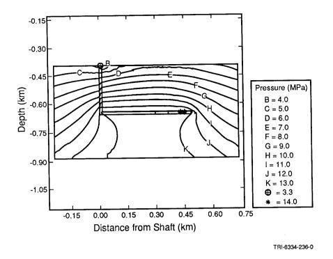
Figure 3-19. Pressure Contours for SUTRA, Set II, Case IB, Degraded Properties and Boundary Conditions Interpolated from Large-Scale Simulations at 10,000 Yr. (Figure 3-12 shows corresponding, large-scale simulations.)
