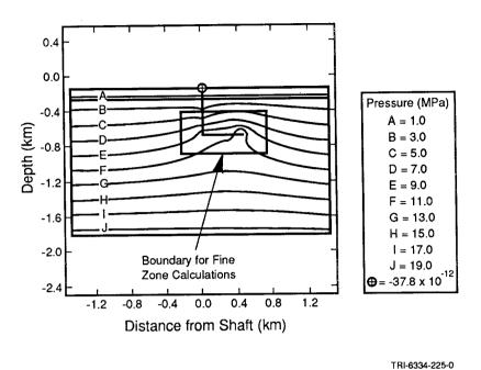
Figure 3-9. Pressure Contours for Large-Scale SUTRA Calculations Used to Provide Boundary Conditions for Set II, Case IA (Steady State).
