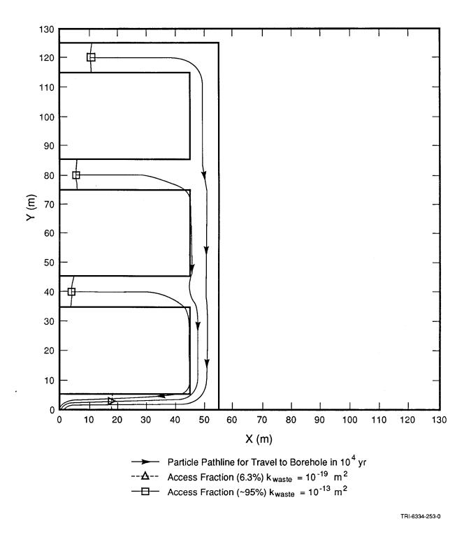
Figure 4-25. Fraction of Waste Accessed in 10,000 Yr with Waste Permeabilities of  $10^{-13}$  and  $10^{-19}$  m<sup>2</sup>, and Capacitance of 5.1 x  $10^{-9}$  Pa<sup>-1</sup>.
