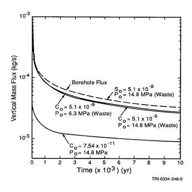
Figure 4-22. Vertical Mass Flux as a Function of Time as Calculated by Cylindrical SUTRA Model.
