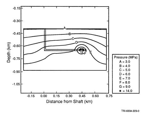
Figure 3-7. Pressure Contours for SUTRA Calculation Set I, Case IA, Showing Hydrostatic Boundary Condition Edge Effects.
