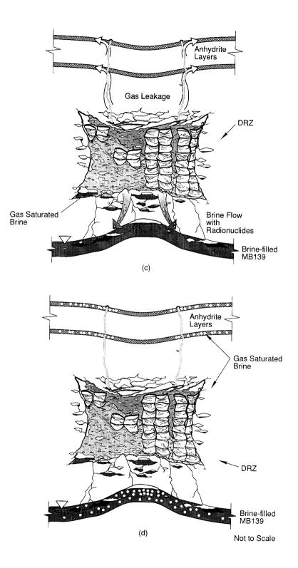
Figure 2-1. Hypothesized Episodes in Disposal Area Leading to Undisturbed Conditions. (Continued) This drawing shows (c) gas generation, brine outflow, and room expansion, and (d) undisturbed conditions with gas-filled room surrounded by gas-saturated brine.
