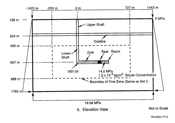
Figure 3-3. Schematic and Boundary Conditions for Large-Scale SUTRA Calculations Used to Generate Boundary Conditions for Embedded Fine Zone (Set II).
