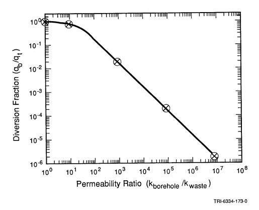
Figure 4-16. Steady-State Diversion Fraction versus Borehole/Waste Permeability Ratio.
