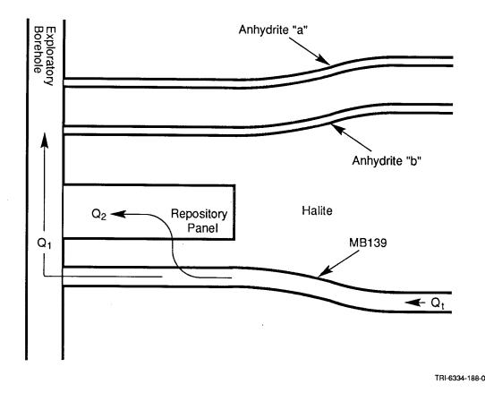
Figure 4-8. Schematic Diagram of Stratigraphy Surrounding Repository Panel Showing Potential Discharge Paths to an Exploratory Borehole.
