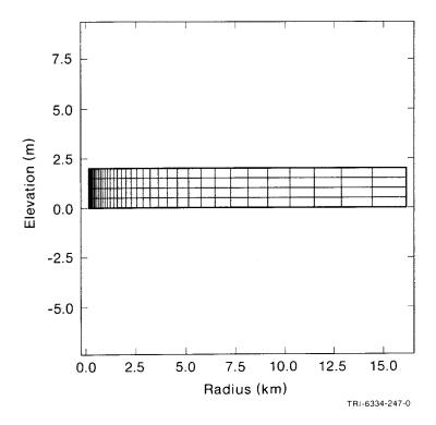
Figure 4-20. Mesh for Cylindrical Model of Room with Gas for Evaluating Characteristic Depressurization Times.
