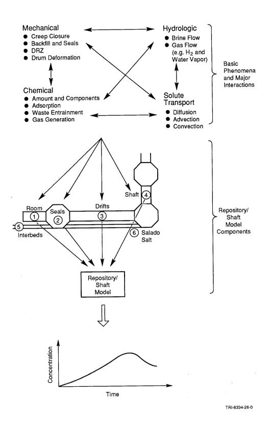
Figure 1-12. Basic Phenomena, Major Interactions, and Components of the Repository/Shaft Model (after Rechard, 1989).
