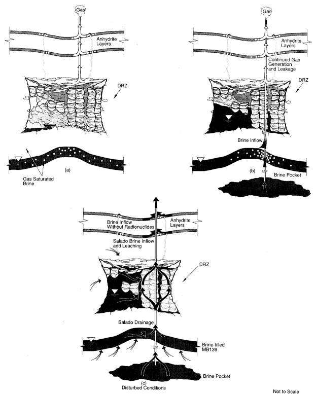
Figure 2-2. Hypothesized Episodes in Disposal Area After Human Intrusion. This drawing shows (a) initial room gas depressurization when penetrated by exploratory borehole, (b) final gas and brine depressurization as borehole seals degrade, and (c) brine flow through borehole to Culebra Dolomite.
