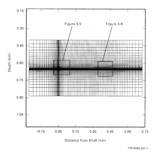
Figure 3-4. Mesh of SUTRA Calculation of Undisturbed Repository/Shaft System for Sets I and II (Fine Mesh). Regions illustrated in Figures 3-5 and 3-6 are shown.
